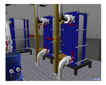
The highly realistic 3-D modelling and zoom technique make it very easy to access any part of the engine room and to open and close valves, set the position of switches, push-buttons etc.
